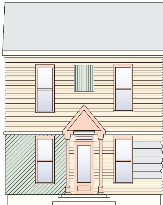
Figure 3: Illustration showing an inappropriate combination of siding.
